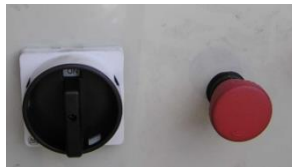
Fig. 3. Safety switch and emergency stop (red)
